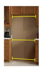
Measure the depth of the counter on each side of the refrigerator.
